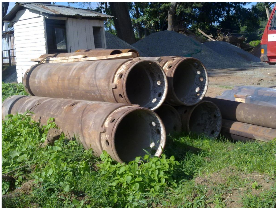
Double Wall Casings ( diameter 620, 880, 1000, & 1200 mm )
