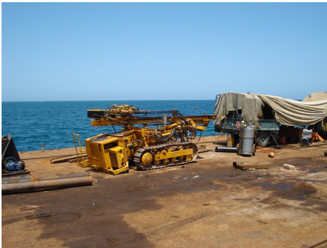
Klemm Deep Driller (For Geotechnical Investigation & Anchoring)
