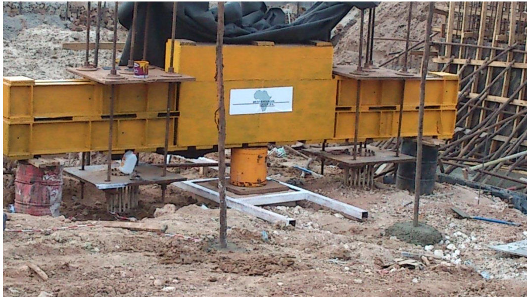
Pile Load Testing (up to 600tons at NHC Plot 300 Project, Dar Es Salaam Tanzania)
