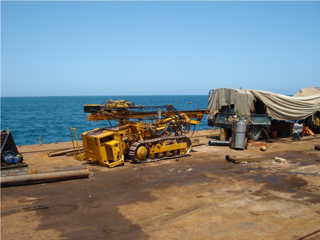
Klemm Deep Driller (For Geotechnical Investigation & Anchoring)
