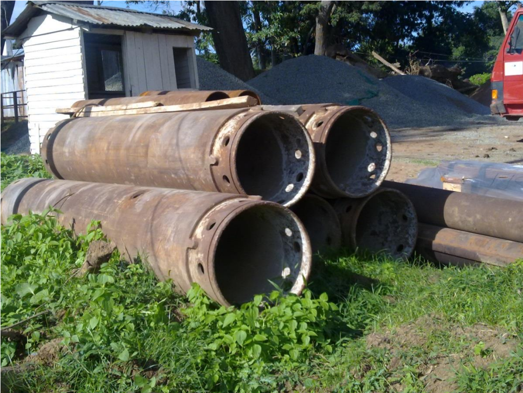
Double Wall Casings ( diameter 620, 880, 1000, & 1200 mm )
