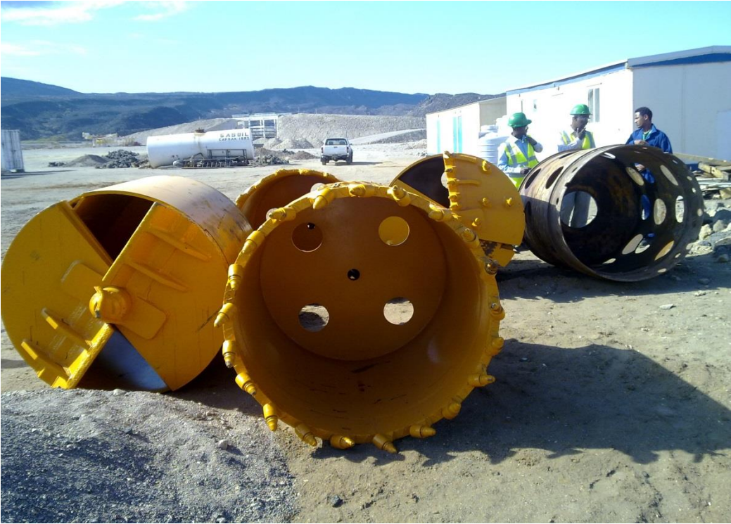
Diff. Big Diameter Drilling Tools ( diameter 620, 880, 1000 & 1200 mm )
