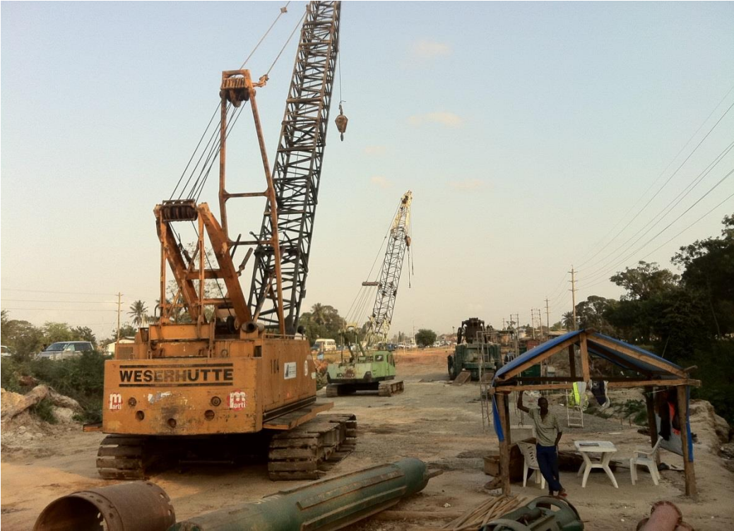
67 tons Crawler Crane Weserhütte on Bridge Project in Dar Es Salaam, Tanzania
